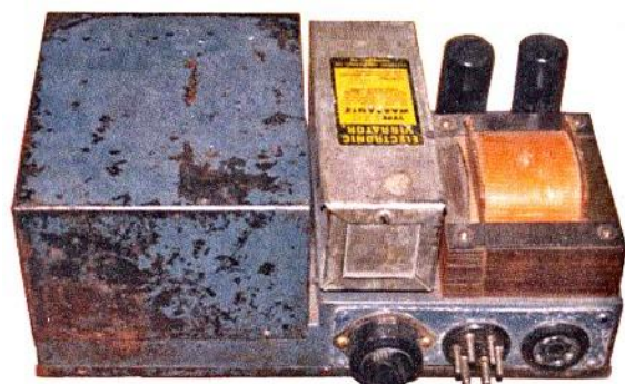
AC mains and 6V DC power unit of 'Lagercrantz 1'.
